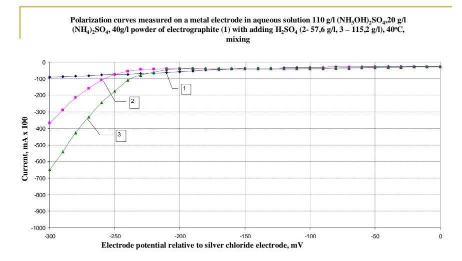
The operation of the system is based on the relationship between redox currents on the polarized electrode in potentiodynamic mode and the of sulfuric acid concentration.
