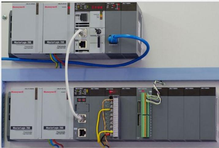
Controller with 2 input-output units
